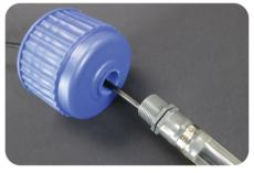
5. Insert vent hose thru the center of the lid
